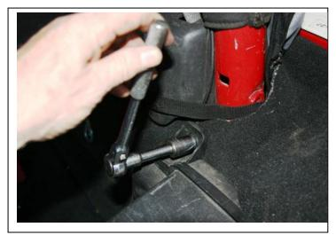
3. For fitment, place the large bracket in the slit so you get the location and angle right, then carefully pull the carpet back and mark the location of the bracket. The rear edge of the bracket should just touch the rubber tail gate seal.
