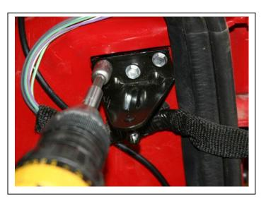
5. Snap on the small end of the gas spring. Open the tailgate all the way to the stop so you can position the small bracket. You will be installing that bracket so the spring pushes the tailgate all the way to the Jeep's stop.
