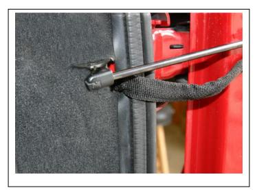
6. With the tailgate pushed (by you) against the Jeep's stop, mark the location of the outer (small) bracket. The outermost screw should be 2 ¼ inches from the top of the tail gate. The other screw should be about 3/8" lower. The one you see here is only ¼" lower. You will be able to easily see where it goes by putting in the outer screw first, then aligning the bracket with the slanted spring.
