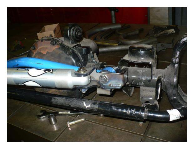
5. Using a drill motor with a 3/8" or 9.5mm drill bit, drill the side and bottom of the factory track bar bracket to match the holes in the new track bar relocation bracket. The side hole is difficult to get a strait shot with the drill; you may have to drill down at a slight angle. (Note the picture below is an older style prototype part, the production part looks different but utilizes the same mounting holes.)
