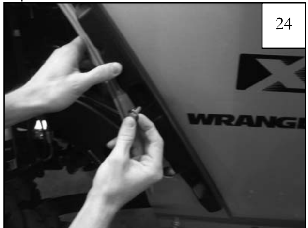
Step 2 Slide a .700" Washer onto 5/16" Hex Head Bolt. Insert a bolt/washer assembly through inner flare piece and fender and secure with 5/16" Nylok Nut. Start the bolts but do not tighten.
