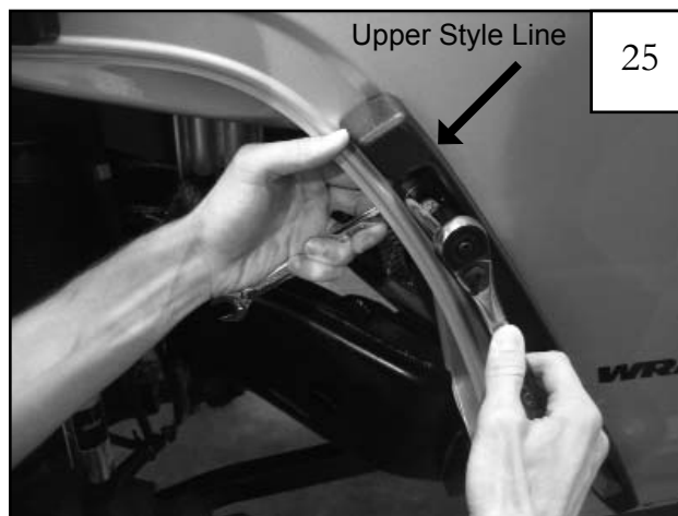
Step 3 Using a 1/2" socket wrench and a 1/2" wrench, tighten all bolts until inner piece is snug against fender. Do not overtighten: see step 21. Inner piece should rest along upper style line of sheet metal radius and not below it: see step 22.
