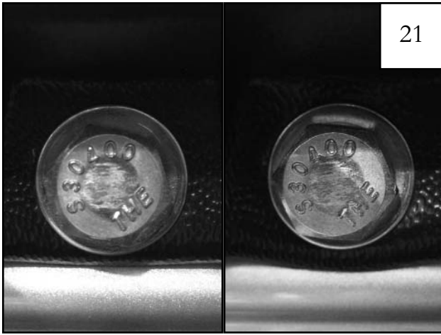
Bolt on left: Properly tightened; lower edge of inner piece runs straight Bolt on right: Overtightened; lower edge of inner piece bows down; if accidentally overtightened, remove inner piece completely before reinstalling
