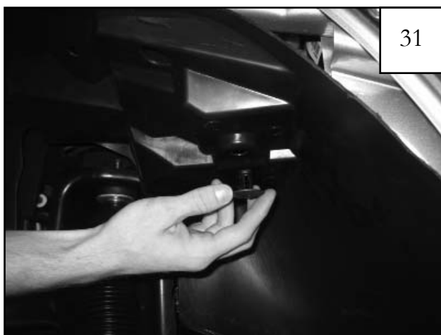
Reinstall factory fastener removed in Step 2 in location shown. 2007-2010 model years, fastener is a plastic thread engager. 2011-newer model years, fastener is a 10mm bolt.
