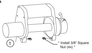
Note: If installing winch, rest winch in place, do not install bolts (item J). It will be necessary to move winch (side to side) to install bumper hardware.
