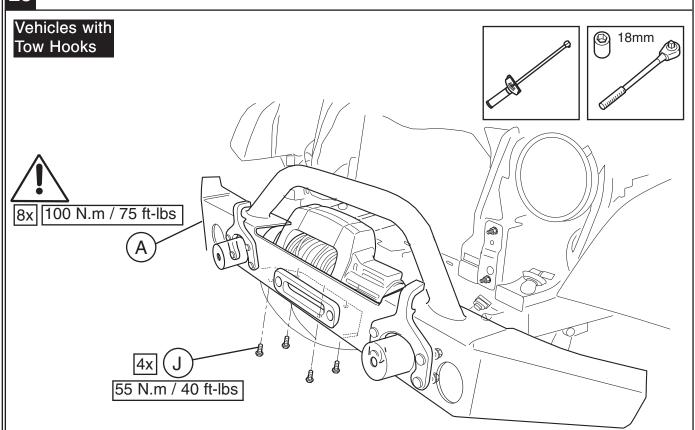
After leveling the bumper for best appearance, torque hardware as shown 8 places.
