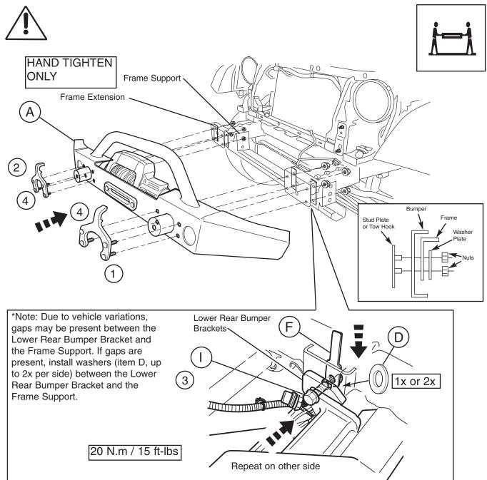
Rotate Bumper under frame extension to align lower rear bumper bracket slots to frame support hole (see frame 7) and then loosely install two tow hooks with nuts and washer plates (removed in step 5). Now loosely install bolts (item I) to handle nuts (item F). Due to vehicle variations, washers (item D) are supplied to eliminate gaps.
