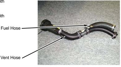
f. Install fuel filler assembly on fuel tank with two clamps.
