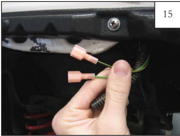
Install a Male Wire Connector to the end of each factory side marker light wires and secure by pressing firmly with a wire crimp.
