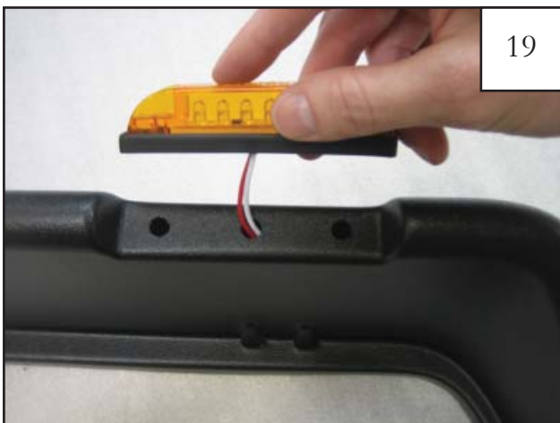
Position the supplied side marker light onto the outer flare piece, threading the wires through the center predrilled hole.
