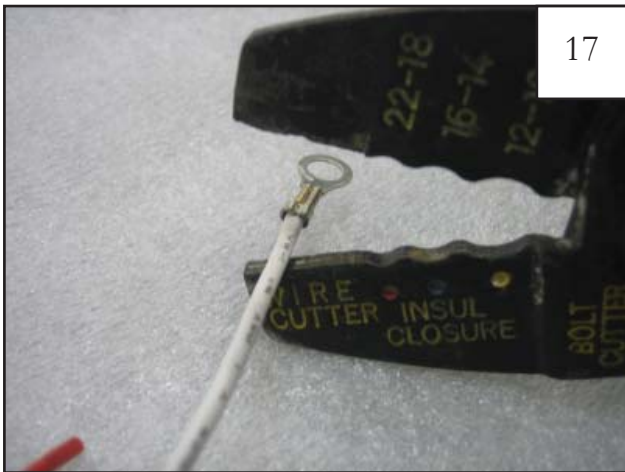
Use wire cutters to cut the eyelet from the supplied side marker light.
