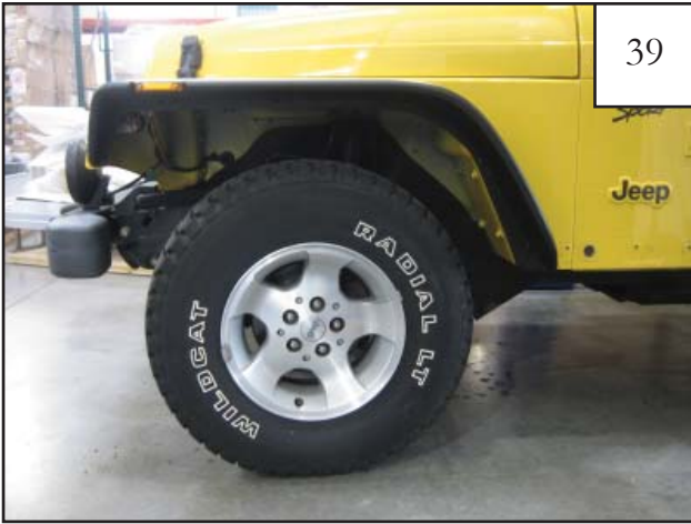
Completed front driver's side flare installation.
