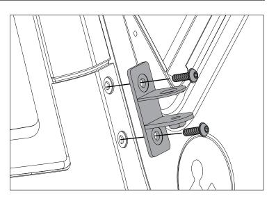
3. Attach Arm to Bushing. Using Thumb Screw, loosely install Bushing and Arm into Mounting Bracket.
