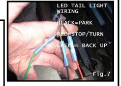
Wiring for the LED Tail Light is as follows:
