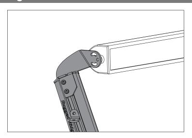
5. Remove Wire Cover from A-pillar Assembly. Create a small cutout at top of Wire Cover for wire routing. Cut out holes marked in Step 3.
