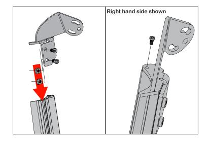
2. Using T40 Torx wrench, remove two upper OE bolts on windshield brackets. Loosely attach A-Pillar Covers using previously removed OE bolts.
