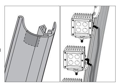
6. Attach Lower Cap to A-Pillar Cover using M8 Bolt and M8 Square Nuts.
