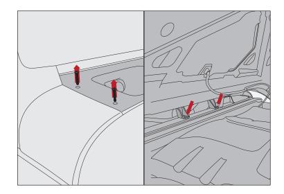
10. Position Light Bar Assembly on factory windshield bracket and reattach Light Bar Assembly using OE bolts.
