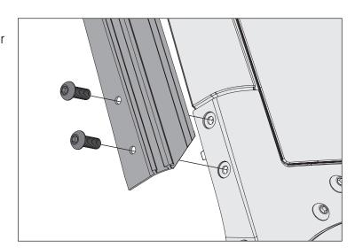
3. Attach A-Pillar Bracket using M8 Bolt and Square Nut in A-pillar Cover's channel. Attach accessory to A-Pillar Bracket. Align accessory per personal preference. To allow easier installation of Lower Caps, remove A-pillar Assembly from vehicle.
