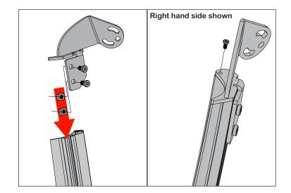
3. Using T40 Torx wrench, remove two upper OE bolts on windshield brackets. Loosely attach A-Pillar Covers using previously removed OE bolts.
