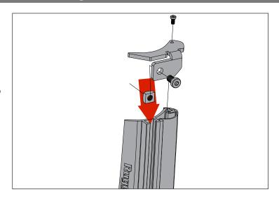
2. Construct A-pillar Assembly by attaching LED Bracket to the top of A-Pillar Covers using M8 Bolt and M8 Square Nut. Slide M8 Square Nut down channel on A-Pillar Covers. Using M4 Bolt, secure LED Bracket to top of A-Pillar Cover.
