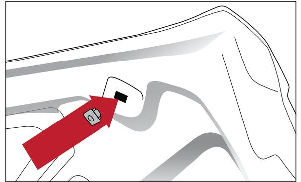
2. Remove red protective backing from double sided tape. Install bug deflector. Secure with two washers and two screws into previously plugged holes. Press firmly on taped areas and hold for 60 seconds.
