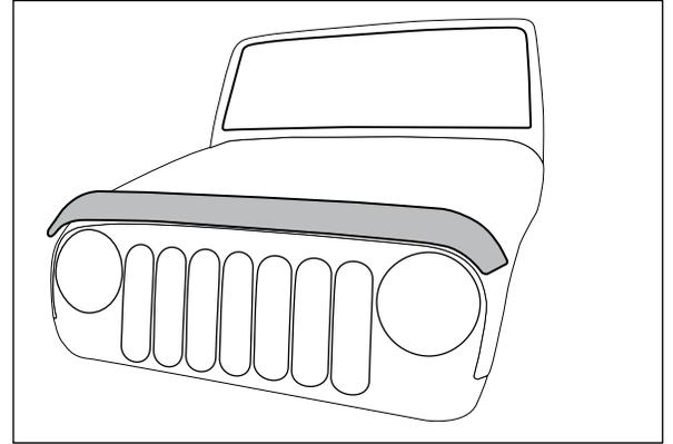
1. Clean and open hood. Test fit bug deflector centrally on hood. Note (2) holes in hood corresponding with two slots in bug deflector. Remove bug deflector. Insert plastic screw plugs into holes previously noted.
