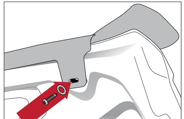
NOTE: Do not use power tools to install this product. Do not overtighten.
