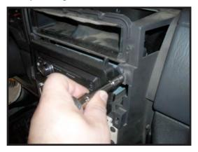
3. Install radio into iVault Radio Mount. Note - the sleeve that comes with the radio is not used. Radio is placed directly into iVault Radio Mount and attached using provided screws. Make sure all wiring is properly connected as per radio manufacturer instructions. Place iVault Radio Mount, with radio, into dash. Fasten to dash with (2) bolts removed in step 2.
