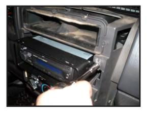
4. Reinstall Radio surround by aligning clips and pushing it into place. Reinstall (2) screws removed in step 1. Press vent cover back into place that was removed in step 1.
