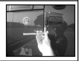
4. Loosely attach Hinge Pin Brackets to Tube Doors using supplied M8 hardware.
