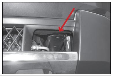
2. Remove plastic splash guard under front bumper cover.
