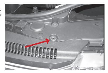
8. Apply a layer of Adhesive Foam Tape to bottom of Driver Side Top Bracket. Place Driver Side Top Bracket on top of washers and bolt to radiator support using factory hex bolt.
