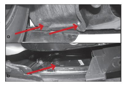
5. Locate the threaded holes in bottom of frame channel. Holding Driver Side Frame Mounting Bracket with mounting tab flat insert through opening and rotate up into position in line with factory threaded holes. Bolt Bracket to frame channel with (2) 10mm x 30mm Hex Bolts, (2) 10mm Large Flat Washers, and (2) 10mm Lock Washers. Do not fully tighten at this time. Repeat for passenger side.
