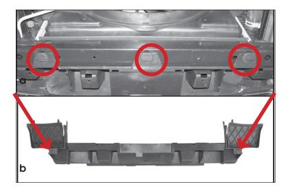
**2014 Models**: The block offs covering openings in bumper are clipped onto back of bumper cover only. Remove hardware at bottom of inner fender panel (a). Release clips behind bumper and remove block off from each opening in bumper cover (b).
