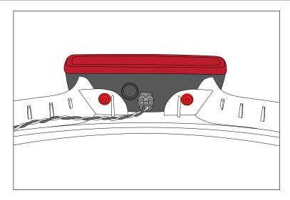
5. Using 13mm socket, remove eight factory bolts securing spare tire mount. Remove wires for third brake light and back up camera.
