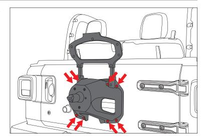
6. Install Wheel Mount using supplied M8 Hex Bolts, Washers, and Spacer Plates on passenger side.
