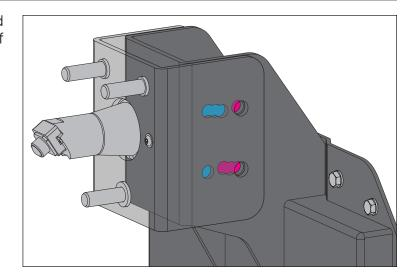
9. Install Camera Shield on factory lug stud assembly.
