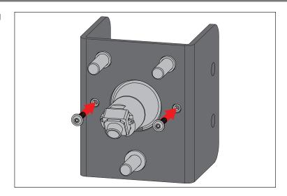
8. Install Stud Plate on Wheel Mount using supplied M12 hardware. Stud Plate can be installed in one of six configurations shown.
