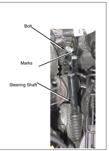
c. Remove bolt and slide u-joint off of steering shaft.
