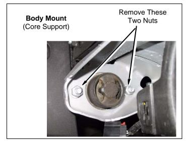
b. Driver Side: Loosen, but DO NOT REMOVE, body mounting bolts. 2 Door - 4 body mount bolts and 4 Door - 5 body mount bolts.
