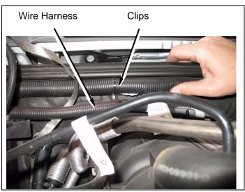
**b.** Install six screw clips along top of grille.
