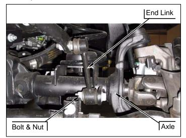
**7.** Using hydraulic floor jack, lower front axle and remove two front coil springs.
