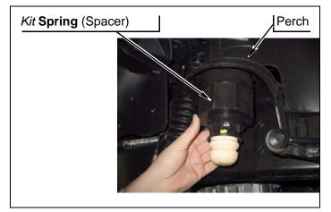
**2.** Install factory spring onto kit **spring** (spacers). DO NOT INSTALL bottom of *kit* **springs** onto axle.
