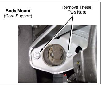
d. Passenger Side: Remove bolt and lower bushing from each cab mount on passenger side. 2
