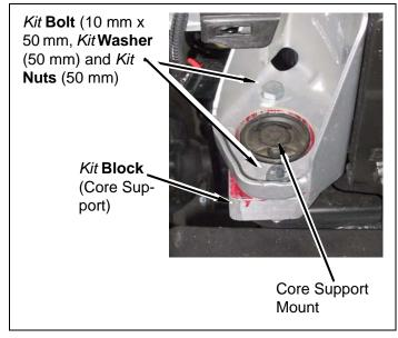
**g.** Install *kit* **blocks** (1" x 3") onto factory body bushings on each body mount.
