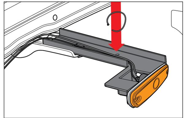
10. Loosely fasten flare to side of fender using two M6 flange bolts and M6 nuts.
