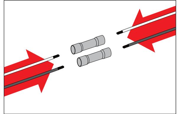
5. Attach and crimp female terminals to wires.
