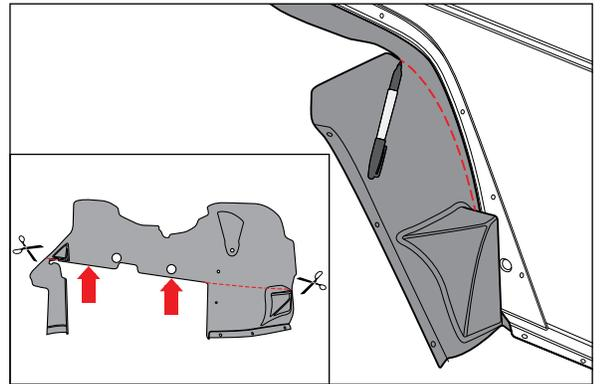
14. If you have a Rugged Ridge Snorkel, mark passenger side wheel liner where indicated. Carefully cut area marked.
