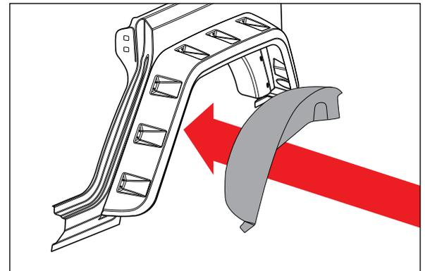
22. Secure wheel liner using M6 flange bolts, 16mm washers, and M6 nuts in locations indicated by **Red Arrows**.
