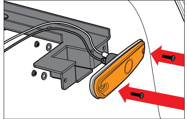
9. Loosely secure wires to support arm with zip tie and uninstall side marker.
