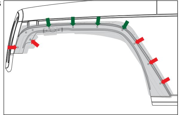
16. Place and position cut front liner in wheel well.
