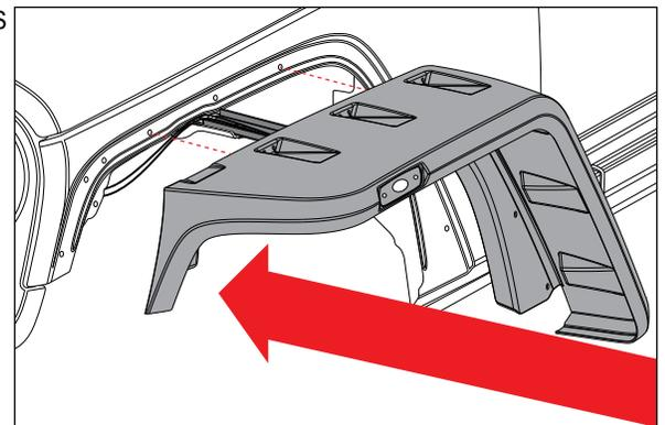
11. Mark your fender using hole shown as guide. Remove fender flare after fender is marked.
