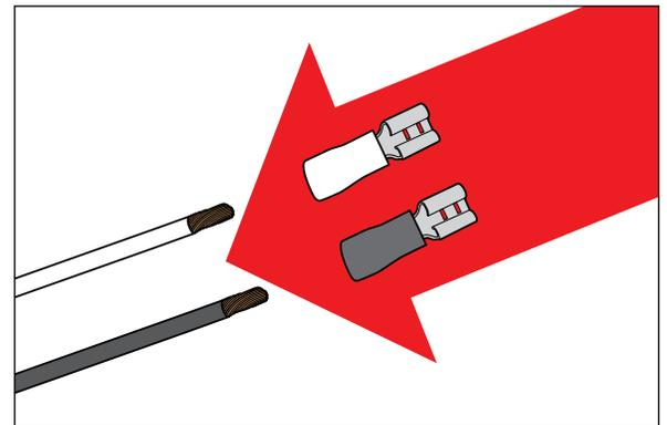
6. Insert female terminals into side marker lights supplied.
