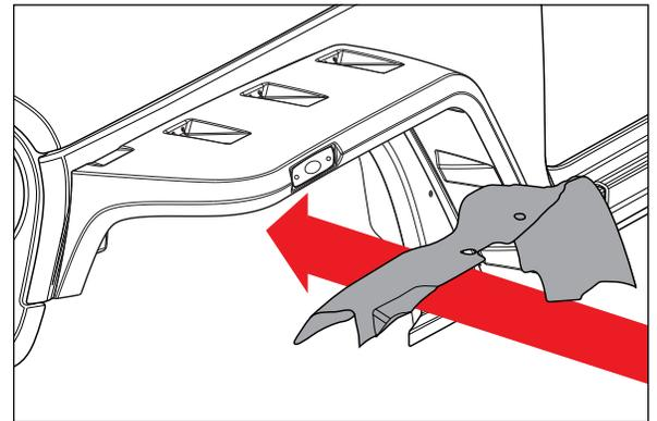
17. Use factory screws previously removed and 45mm washers to secure wheel liner where **Red Arrows** indicate.
