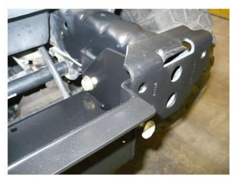
11. Install the frame nut plates to the side of the winch mounting plate. Use the ½ x 1 bolts with flat washers. The nut plates are R and L so install them as shown. Leave these bolts loose until you install and tighten the bumper bolts.
