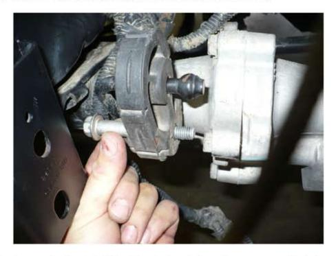
Loosen the front stabilizer bar retainer bolt on the passenger side to lower the stabilizer bar enough to rotate the disconnecting stabilizer bar unit up and in front of the radiator. You will need to notch the lower radiator plastic cover to clear the electrical plug.
