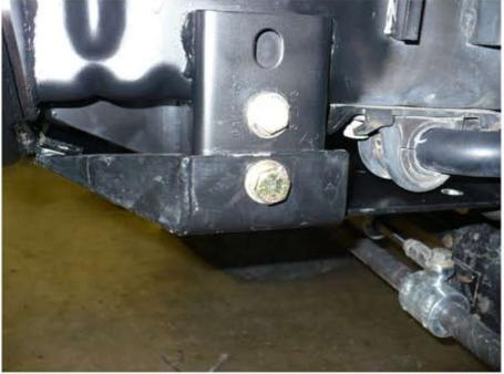
16. Position the rear stabilizer bar bolt spacer between the skid plate and stabilizer clamp. Loosely install the new M10 x 90 bolts and use a 3/8" flat washer. Do not tighten yet.
