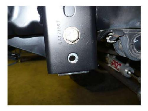
15. Position the skid plate over the frame side brackets and under the tabs on the bumper, loosely install the ½ x 1 bolts and washers thru the frame side brackets into the lower hole in the nut tab.
