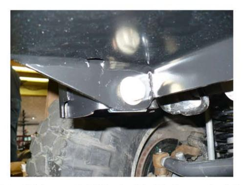
12. Install the bumper with the <sup>1</sup>/<sub>2</sub>" carriage bolts. The 4 longer carriage bolts go thru the inner holes and thru the winch mount. The 2 shorter ones go in the outer bumper holes. Use a flat washer and a lock nut. Tighten the bumper bolts first then the winch mount side bolts to 60 ft-lbs.
