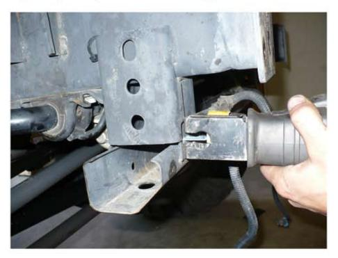
4. Remove the rear sway bar mounting bushing bolt on both sides.
