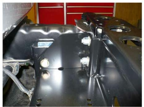
13. Install the winch and fairlead at this time before the skid plate is installed. A hawse type fairlead is required; a roller fairlead does not fit in the bumper. The hook on the front of the winch mount is provided to hold the hook when the cable is spooled in, it is not a tow or recovery point.
