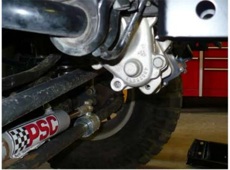
5. Remove the bottom rear bolt in the disconnecting stabilizer bar housing as shown
