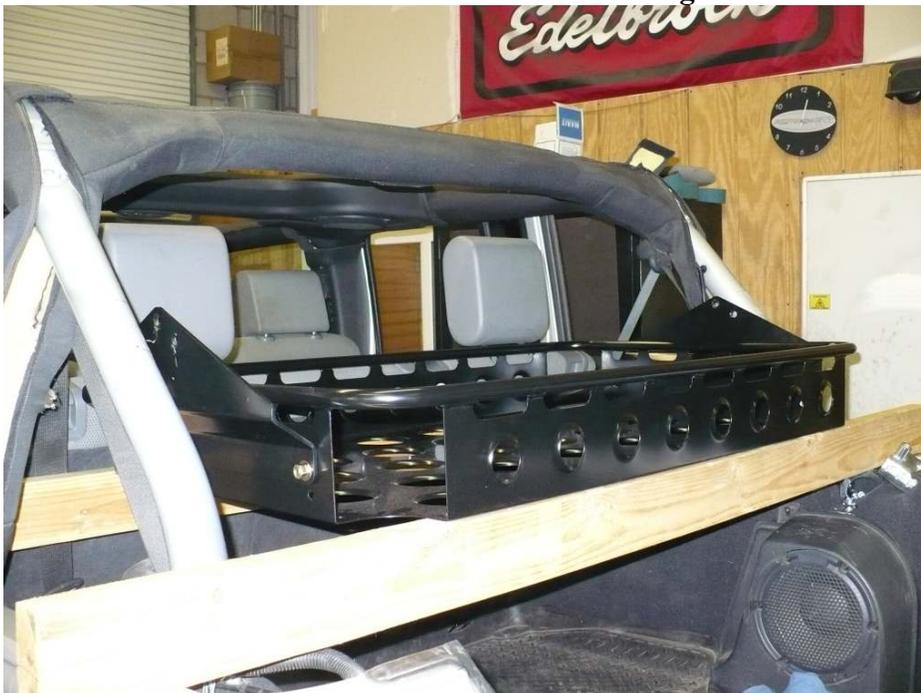
6. With the side mounting brackets installed, first place two 2 x 4" x 5 1/2' pieces of wood across the rear tub of the JK. **See Figure 1**. Position the wood so the rack rests on the flat surface of the rack, do not place on flared holes. This will level the rack to the preferred installation height.
