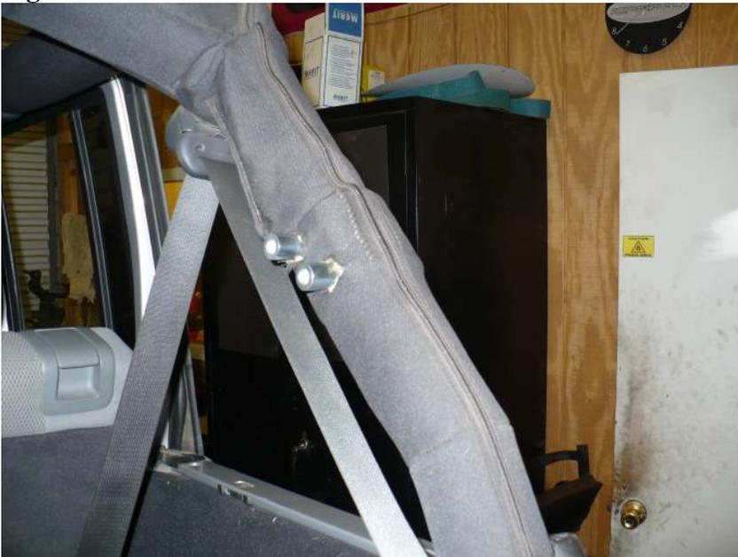
22. Reinstall the rack using the (4) 7/16" mounting bolts and lock washers. Torque the bolts to 40 ft-lbs.
