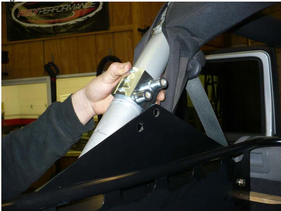
10. Align the tube clamp and rack side mounting plate holes. Install the (2) 7/16 x 1" bolts and a 7/16" lock washer under the head of each bolt. Tighten to finger tight. See **Figure 3**
