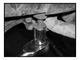
3. Remove two side steering box bolts as shown. These holes will be used to mount the steering box skid plate.
