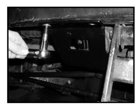
6. Insert top rear steering box bolt back into its proper position and tighten. The installation of your YJ Steering Skid Plate is now complete!
