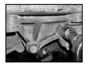
4. Place skid plate in location to line up with the two side steering box holes. Use the supplied 12mm hardware to mount skid plate. Do not use lock washers at this time. Hand tighten only as the skid plate will have to be removed. Mark the two front mounting holes on the bottom of the bumper. Remove skid plate and drill holes to 3/8" diameter.
