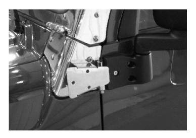
Carefully remove the two bolts on the lower part of the windshield hinge. Position and mount the relocation bracket using the 5/16" bolts provided. Remove the factory mirror from the door and mount the mirror to the bracket using ½"-20nc bolts and nuts provided. Make sure all bolts are securely tightened. With help adjust the mirrors to your needs. We recommend that you use anti sieze on all threads of the stainless bolts provided with your parts.
