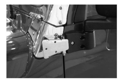
Carefully remove the two bolts on the lower part of the windshield hinge. Position and mount the relocation bracket using the 5/16" bolts provided. Remove the factory mirror from the door and mount the mirror to the bracket using \(^1/4\)"-20nc bolts and nuts provided. Make sure all bolts are securely tightened. With help adjust the mirrors to your needs. We recommend that you use anti sieze on all threads of the stainless bolts provided with your parts.
