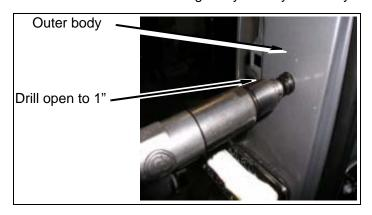
c. Drill out remaining inner body layer to 1/2"
