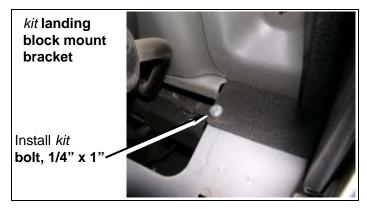
e. From underside of body center punch and drill upper hole into body with 1/8" pilot drill.
