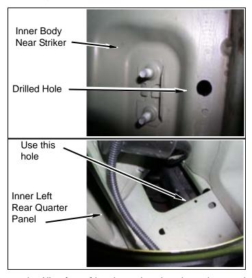
d. Align foot of bracket to location shown here and install *kit* **bolt** (1/4" x 1") with **hardware**.
