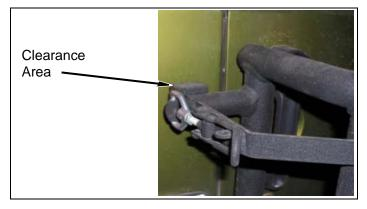
e. Adjust tail gate for proper closing and tighten all remaining bolts inside body. Reinstall tail gate hinge plastic covers.
