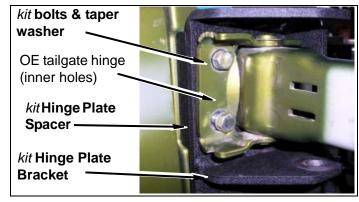
b. On outer hole of top hinge, Install using one *kit* **bolt** (8mm-1.25 x 60mm) with **taper washers** (8mm). Do not tighten at this time.
