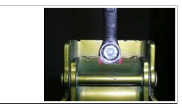
6. Install tailgate hinges, spacers, hinge plate spacers and hinge plate to jeep body. Make sure rounded edges of hinge spacer blocks are toward body.
