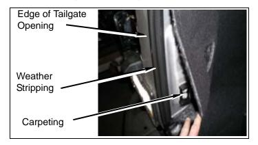
b. Use stencil from the back of these instructions or measure from inner lower corner of body up 4" for first hole location and 11" for second hole location center punch and drill 1/2" hole on each as shown.
