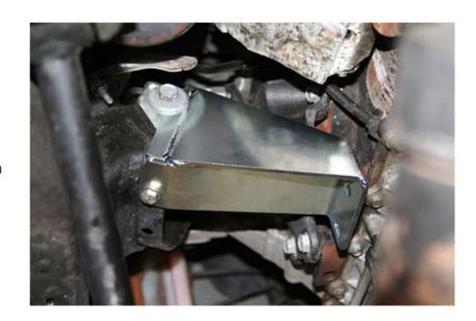
9. Install the driver side frame brace to the frame bracket; the driver side is the shorter of the two. There is no top or bottom and can be installed in either direction. Use the supplied 3/8 bolts, flat washers and lock washers. Leave these bolts loose until all the other pieces are installed.
