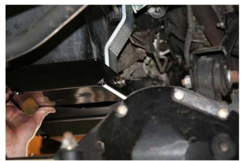
11. Install the passenger side frame brace as shown with the larger hole in the top. Use a ½" bolt with a flat washer and flange nut on the top and two 3/8" bolt with a lock nut and flat washer on the bottom.
