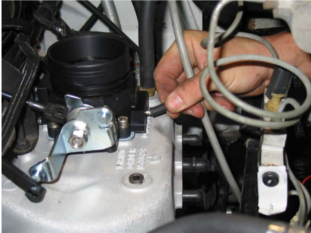
Figure 4.4 PERFECT MAP sensor vacuum hose connection
