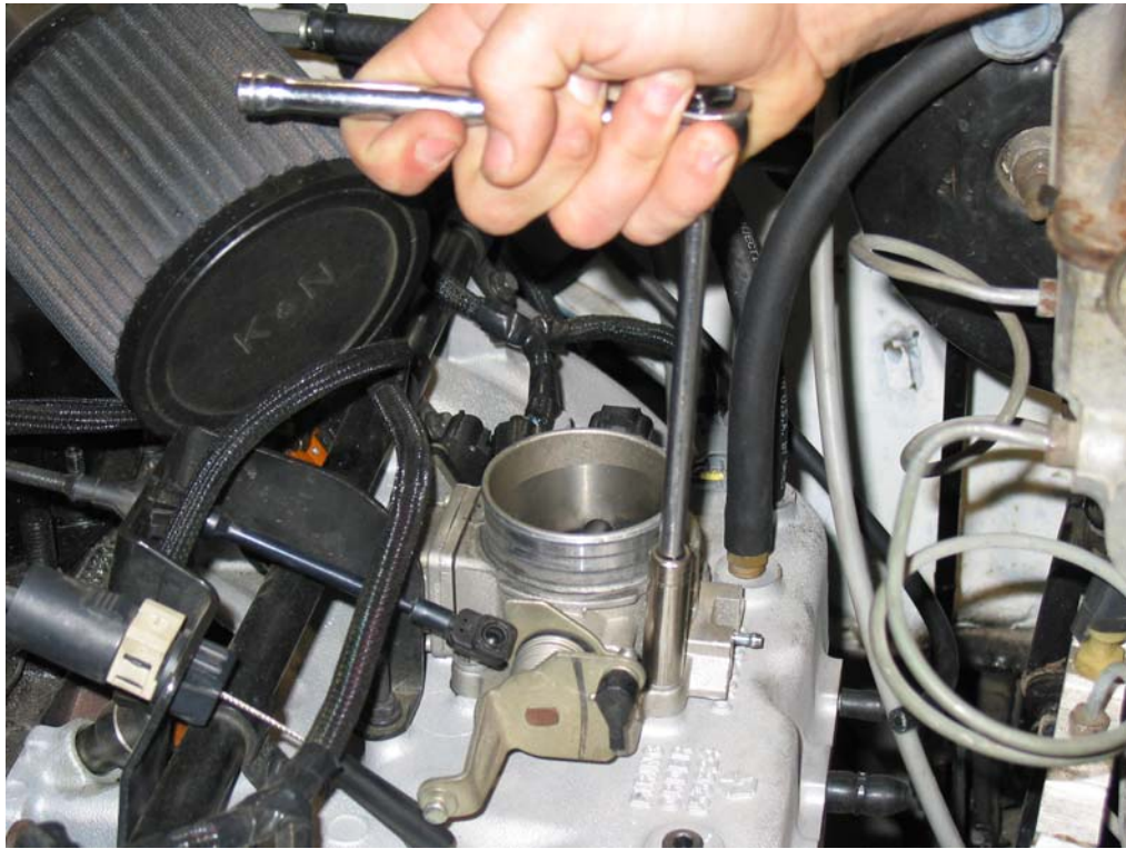
Figure 3-4 Removal of the Throttle Body and bolts.
