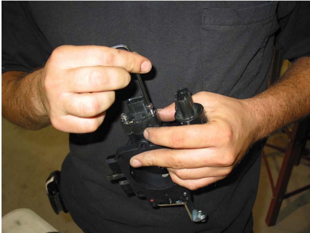
Figure 3.8 Installing the Throttle Position Sensor (TPS)
