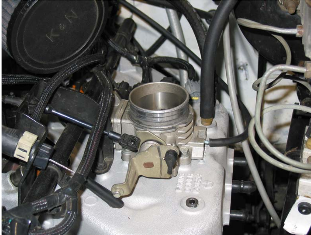
Figure 3-2 Throttle/Kickdown/Cruise Control Cable removal
