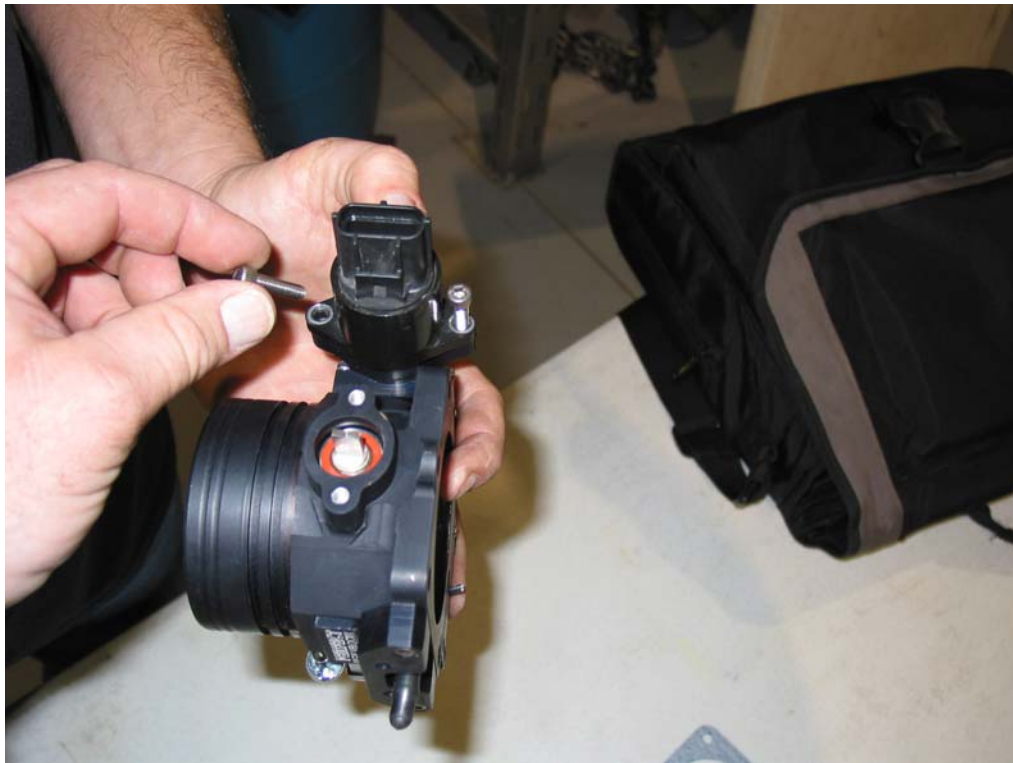
Figure 3.7 Installing the Idle Air Control (IAC) Motor
