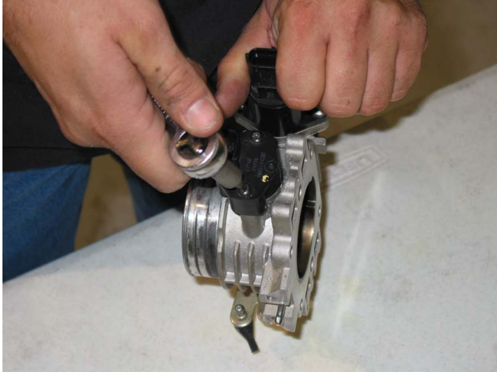
Figure 3.5 TPS and IAC motor removal
