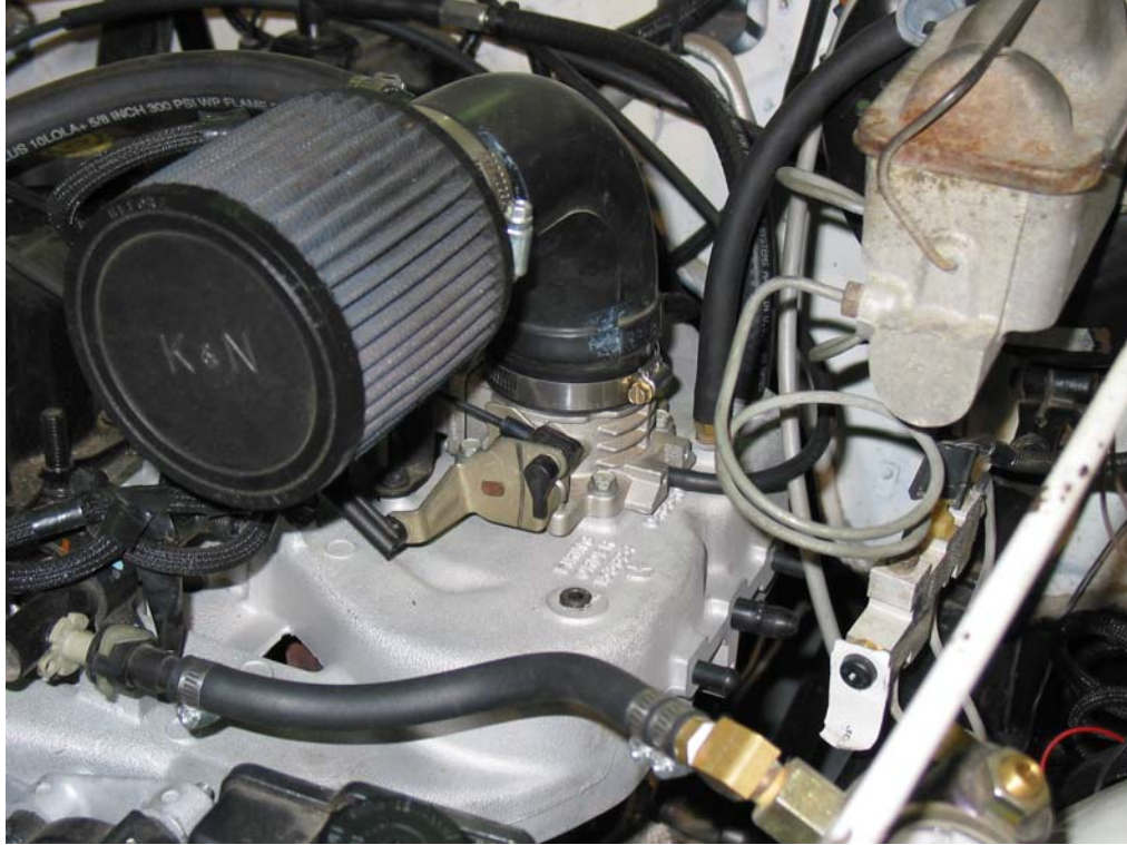
Figure 3-1 Air Filter and Intake Tube Removal
