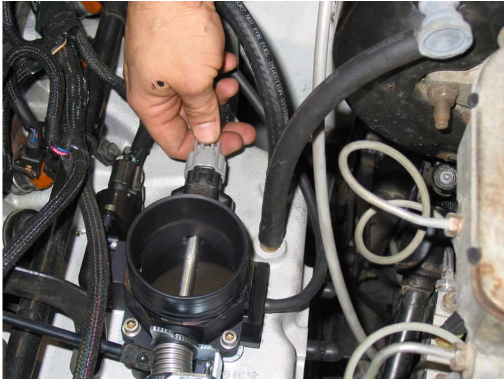
Figure 4.2 Connecting Throttle Position Sensor (TPS)
