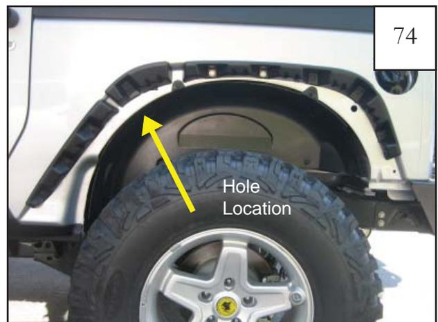
Secure inner piece D9 (and P9 for passenger side installation) to the sheet metal using the following **2 STEPS: Step 1** Position inner piece on fender, aligning with existing factory hole in sheet metal.
