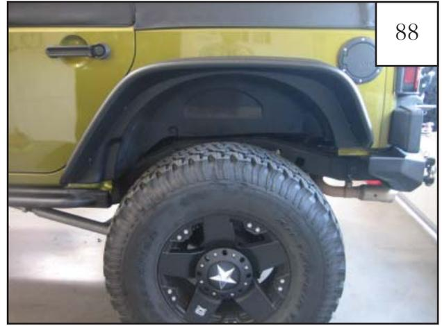
Completed rear driver's side flare installation.
