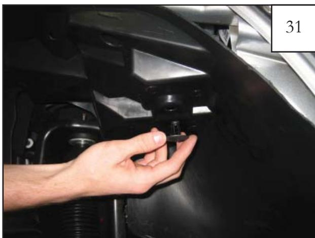
Reinstall factory plastic thread engager in location shown in picture.
