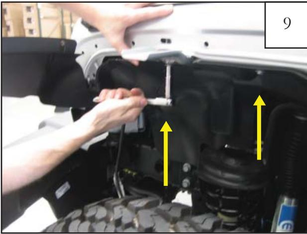
Reinstall the splash shield, in preparation for marking before cutting, using supplied 1.25" Washer on factory bolt/washer assembly and reinstall through factory threads in sheet metal (2 locations).
