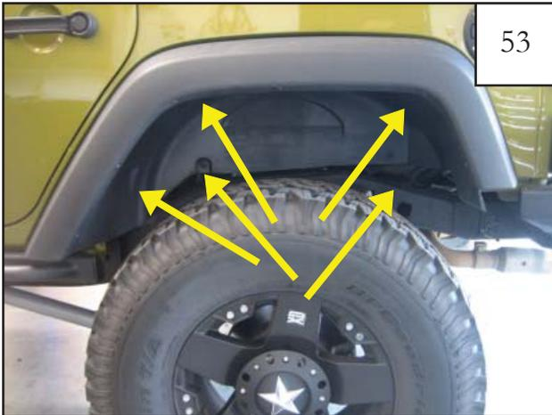
Using a pry tool, pliers, or flat head screwdriver, remove four plastic fasteners from inside of splash shield.
