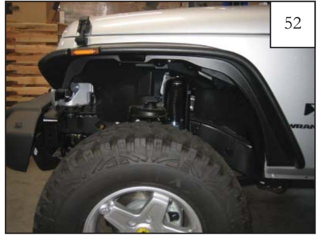
Completed front driver's side flare installation.
