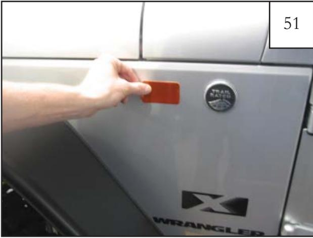
Attach one side reflex reflector to the side of the vehicle by peeling off the adhesive backing and pressing it firmly onto the cleaned vehicle surface. *NOTE: Once reflector has adhered it cannot be repositioned.*
