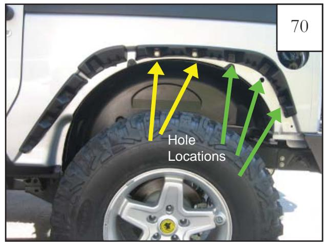
Secure inner piece D6 (and P6 for passenger side installation) to the sheet metal using the following **4 STEPS: Step 1** Position inner piece on fender, aligning with existing factory holes in sheet metal.
