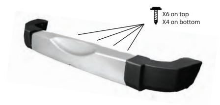
Step 2. Place the cover over the center section of the bumper. Using light pressure hold the cover flush against the bumper. Use the supplied self-tapping screws to attach the cover. Install (6) screws top and (4) screws bottom in the pre-drilled holes in the cover. Re-install the bumper onto the vehicle.
