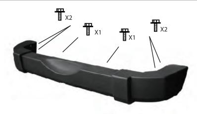
Step 1. Remove the rear bumper. Remove the (6) bolts from the back of the bumper as shown. There are (2) bolts holding each side of the bumper to the frame and (2) in the center of the bumper. Do not discard the bolts, they will be used to re-attach the bumper.
