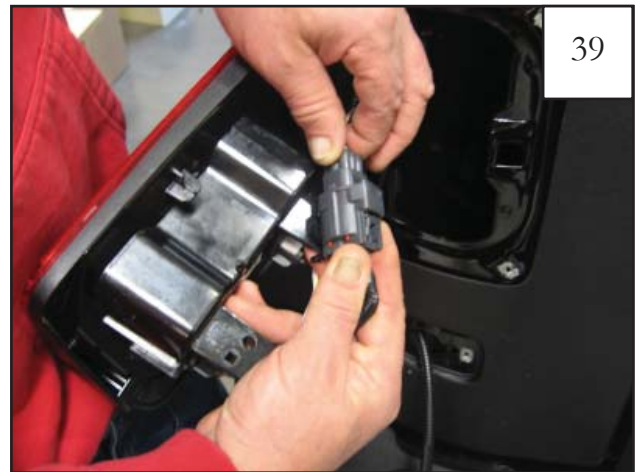
Reconnect light connector of tail light.
