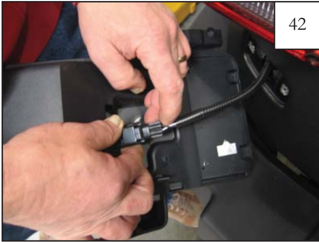
Reconnect light of license plate frame.
