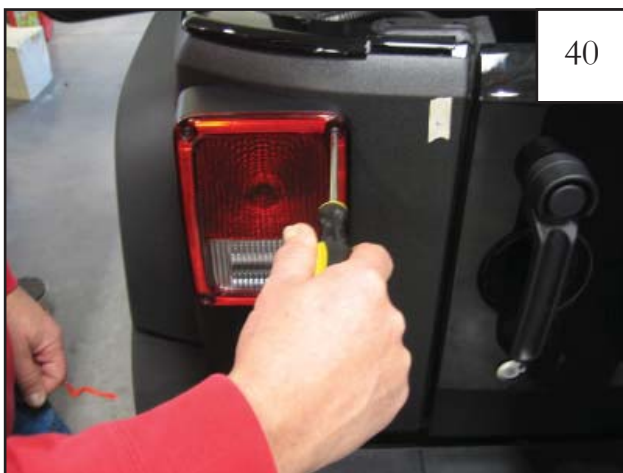
Using a #2 Phillips screwdriver, reinstall tail light.
