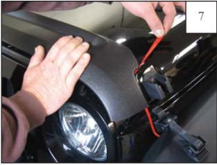
Take the tab of the remaining 1/2" tape strip and pull tape liner. While pulling liner, press on part as was done for first strip of tape liner. NOTE: Take care not to catch tape liner on other piece of tape and accidentally pull its liner off as well.
