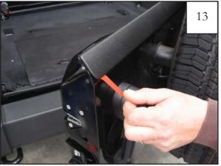
Pull liner of lower 1/2" tape strip. Press down on entire length of part again applying 30 PSI to the taped areas. NOTE: The tape reaches maximum adhesive bond after 24 hours of contact. Do not wash vehicle for 24 hours.
