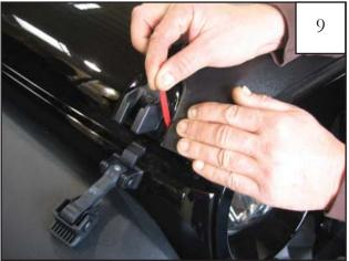
Pull the liner from the lower of the two 1/4" tape pieces on the driver's side of the vehicle.
