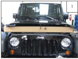
Open front hood. Using box parts came in, prop hood open. Clean all dirt and debris from hood then use supplied alcohol wipe where part will be. NOTE: Temperature should be at least 60°F for proper tape adhesion.
