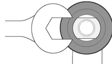
**HINT: Use flat spot on Rod Ends (B) to prevent mounting stud from spinning when tightening 1/2" Flanged Locking Nut (D).**
