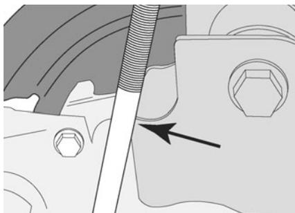
If interference between the control arm bracket and Connecting Rod (A) is discovered, it will be necessary to clearance the bracket per the following instructions.
