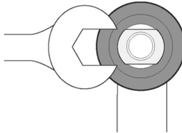
**HINT:** Use flat spot on Rod Ends (B) to prevent mounting stud from spinning when tightening 1/2" Flanged Locking Nut (D).
