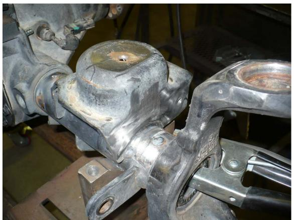
3. Once weld surfaces are prepared, place upper C-gussets in position. There will likely be a slight gap around the ball-joint area; use a C-clamp to tighten the gusset in the proper welding position.
