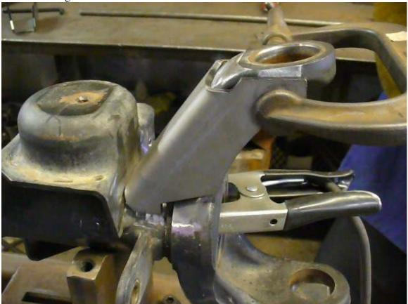
2. Clean the areas to be welded as shown. Take reference of weld photos below to determine exactly which areas will need to be prepared for welding.
