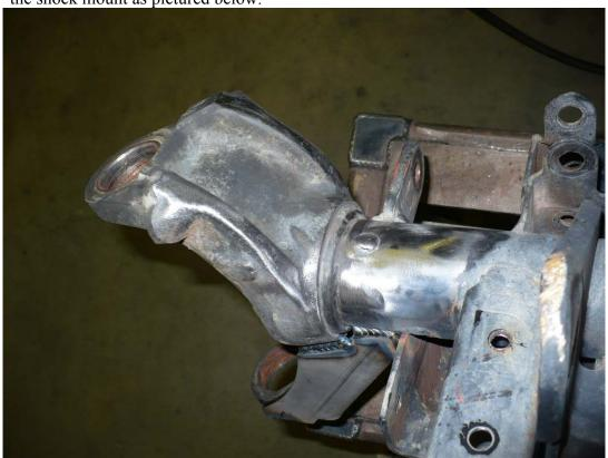
8. Tack the lower C-gusset on in several locations. We recommend tacking at the end of the weld for a clean weld. Once tacked, fully weld as shown in the pictures below.
