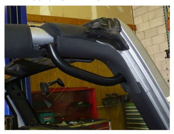
7. Notch the A pillar trim to clear the bottom of the grab handle and install as shown.
