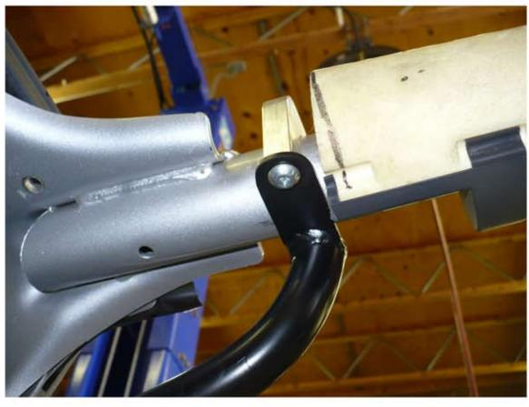
6. You will need to install the grab handle thru the opening in the side bar padding for the soft top door surround. Remove the grab handle and install the side bar padding cover, do not zip the cover until you tighten the grab handle. Torque each bolt to 14 ft-lbs and zip up the padding cover around the grab handle and J hook.
