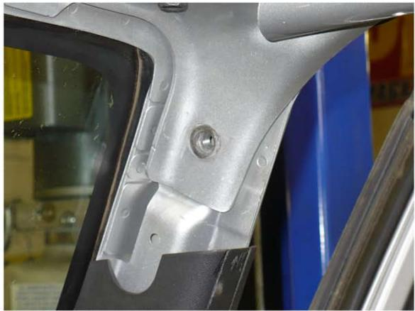
5. Test fit the grab handle to this hole using the factory bolt. The angle bracket end of the grab handle attaches to the windshield and the flat end attaches to the windshield support bar with the J hook just in front of the hole for the soft top door surround. You will have to trim the windshield support bar padding to clear the handle and J hook.
