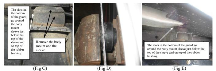
**Step 6:** Cut 3/16" off the top of each of bushings you removed using a hack saw, grinder or some other
