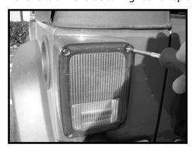
3. Locate the four tail light screws on the passenger side tail light. Remove the top left and bottom right screws. Place the tail light trim piece labeled **R** over the passenger side tail light and replace the screws. Tighten evenly. Be sure the tail light trim is securely fastened to the vehicle before operating.
