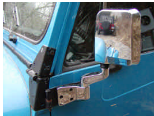
Figure 2. There is no exposed wiring on the outside of the vehicle. This requires drilling holes in the doors and routing wires through the doors. Less exposed wiring provides a cleaner look with less chance of snags.
