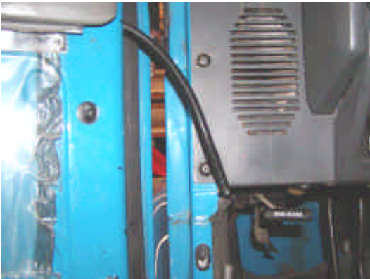
Figure 5. The wires and loom can then be pulled through the door, and the mirror fastened to the door. Be sure to leave the wires long enough to provide for full door movement. Then install the provided male 4-pin plug and terminals. Wiring these plugs
