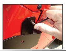
**Step 7.** Place one washer on each bolt, followed by one nut (included). Tighten the nuts snugly, taking care not to over tighten.
