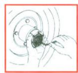
Install clutch assembly. Cross torque allen screws to 14-16 Kp. cm (12-14 in. lbs).
