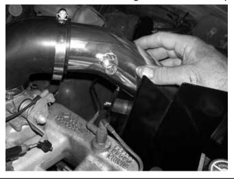
5. Secure intake tube to the rubber isolater mounted on the heat shield with nut and washer.
