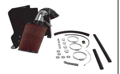
1. Remove original air intake system including air filter housing, air filter, breather hoses, inlet duct. Do not discard hardware, it will be reused.
