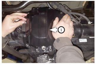
7. Place factory gasket (removed step 4) onto rear differential cover (1). Secure them to rear differential using screws (x2) on both sides as shown.
