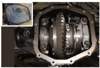
Remove and retain gasket from differential cover; wipe it clean and dry. Then clean mounting surface on front differential.
