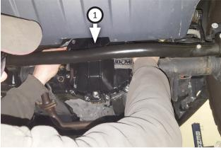
Place factory gasket (removed step 4) onto front differential cover (1). Secure them to front differential using screws (x2) on both sides as shown.
