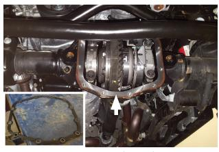
Remove and retain gasket from differential cover; wipe it clean and dry. Then clean mounting surface on front differential.
