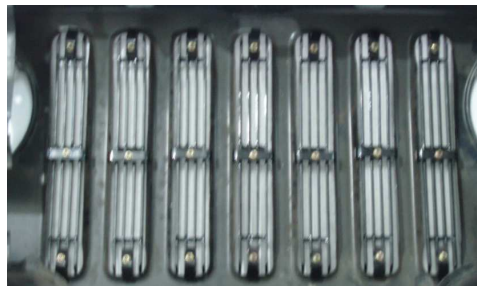
Figure 3 – Rear view of vehicle's shell; Billet Grills attached with Metal Brackets and Flange Nuts
