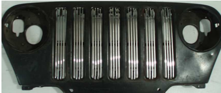
Figure 2 – Front View of positioning lower Billet Grille
