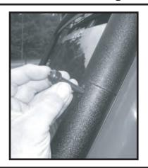
Step 9. Reinstall (2) torx head bolts to front of lower mounting bracket. With all (6) torx head bolts installed tighten securely to windshield frame. Tighten bolts in a clockwise rotation. Tighten M8 Allen head tube bolt. Repeat for other side.
