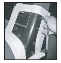
Step 3. If lights are to be installed run required wires through the base of the vehicles windshield. Each lower mounting bracket is supplied with a pre-drilled wiring hole. Fish needed wires through grommet and out the top of the lower mounting tube. It is recommended that disconnects be installed on all wires to allow removal of light bar if needed.
