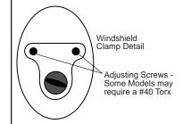
Under most circumstances, the wind-shield of the Wrangler will not require any adjustment. If your Wrangler windshield should require adjustment, this adjustment should be performed only by an authorized automotive mechanic using a special "Tamper-Proof" Torx head tool.
