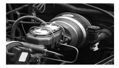
NOTE II : If the vehicle has 4 wheel disc brakes we recommend eliminating or modifying the stock proportioning valve in order to make sure that there is adequate pressure to the rear brakes. You may consider an aftermarket proportioning valve, which is adjustable.
