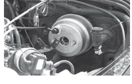
Master Cylinder will require bench bleeding prior to installation. Take care that the rear plug insert of the Master Cylinder does not fall out.
