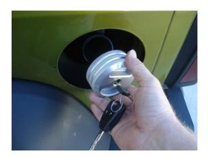
5. Begin to thread cap into gas fill neck in a clockwise direction.
