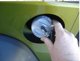
7. Hold cap and turn key clockwise until it stops and then remove key from cap.
