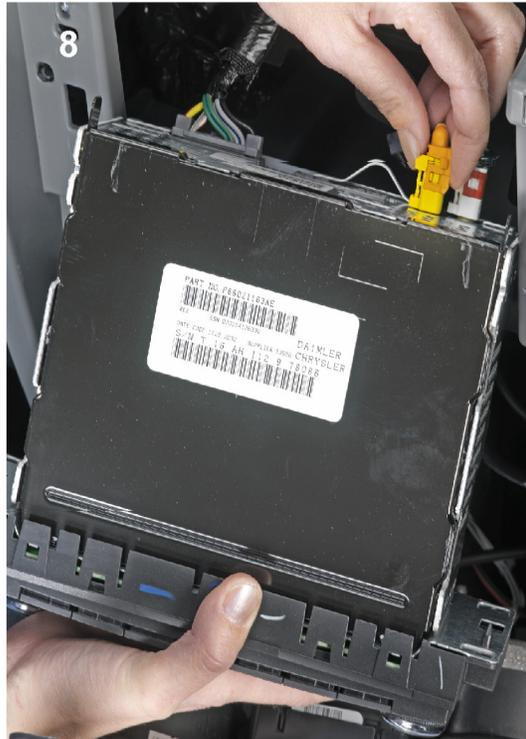
8. Remove the Gray Factory Radio Plug by Squeezing the bottom to release the Plug as shown in picture #9.
