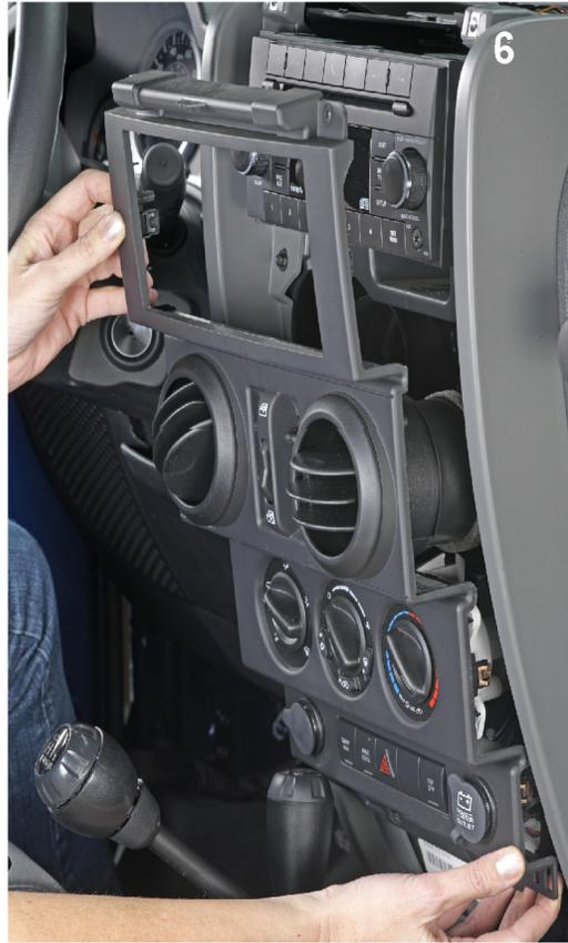
6. Using a 7mm socket remove the 4 screws and slide the Factory Radio out as shown in picture #7.
