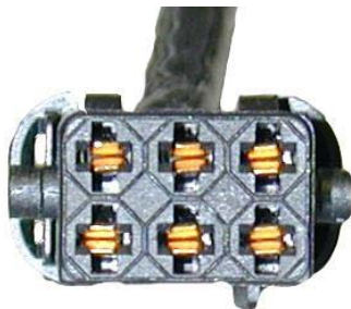
UEGO Sensor connector without latch
