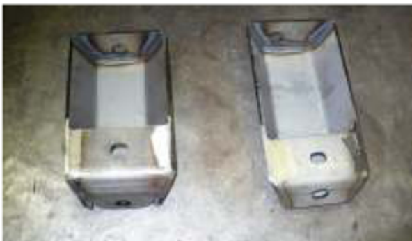
2 door brackets shown front to rear
