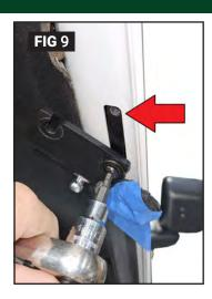
Using a M6 x15 Button Head Bolt and M6 Flat Washer loosely secure Hood Mount Nut Plate to LH (driver's side) Hood Strut Mount (Fig 7). Slide Hood Mount Nut Plate through open slot in hood (Fig 8). Using 4mm Hex Head socket tighten the M6 x15 Button Head Bolt just enough to pull in the Hood mount Nut Plate (<u>red arrow</u>) to hood inner surface. Center threaded hole but <u>Do Not tighten fully</u>. Hood Strut Mount should still move freely (Fig 9).
