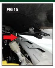
Connect Lift Strut to ball stud attached to LH Hood Strut Mount. Strut main body to be placed towards the top (Hood). A click sound will be heard when properly secured (Fig 13). Connect shaft end of Lift Strut to LH Fender Mount. A click sound will be heard when properly secured (Fig 14). Repeat Step 3 for RH side. Confirm there is no interference as hood is lowered (Fig 15).
