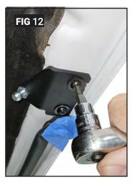
Loosely thread in a M6 x15 Button Head Bolt and M6 Flat Washer into the top hole of the Hood Mount Nut Plate (Fig 10). Rotate LH (driver's side) Hood Strut Mount under M6 x15 Button Head Bolt and Flat washer (Fig 11). Align Hood Strut Mount and secure to vehicle. **Do Not over-tighten** (Fig 12). Repeat step 2 for RH side. Remove masking tape from rubber seal.
