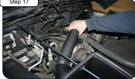
Attach straight coupling with #044 clamps provided on end of intake tube and position to housing and throttle body.
