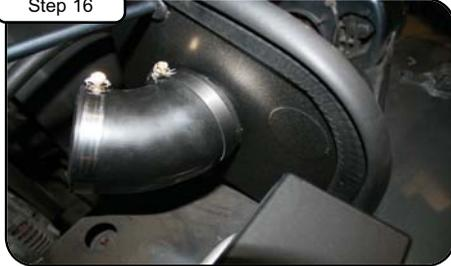
Attach elbow coupling with #048 clamps to housing and position. Do not tighten.
