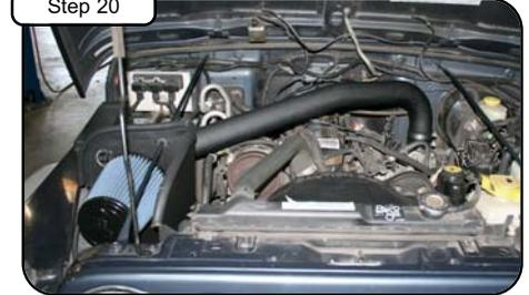
Your installation is now complete. Make sure to check all hoses and tighten any clamps or hardware if necessary. Thank you for choosing aFepower.
