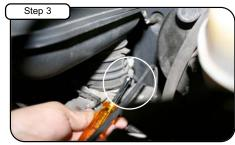
Loosen clamp on throttle body using 5/16" nut driver.
