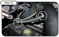
Install 5/8" hose with mini clamps provided and attach to engine and intake tube. Secure mini clamps using 1/4" nut driver.
