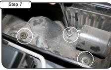
Remove upper half of air box. Loosen the 3 bolts on bottom of air box using 8mm socket or wrench and remove.
