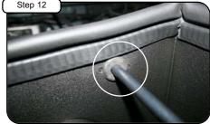
Allign grommet from step 8 and position in hole to prevent core support bracket from vibration.
