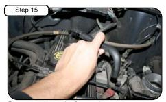
Remove crank case line from engine
