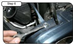
Loosen bolt on core support bracket using 13mm socket or wrench.
