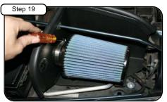
Install air filter and tighten all clamps using 5/16" nut driver. Reconnect battery terminals.
