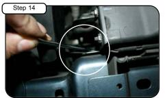
Secure bracket on housing using screw from step 9 using 10mm wrench.
