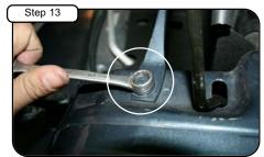
Secure core support bracket using 13mm.
