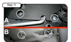
A)Top view: Secure housing using hex screws, fender washers , wavy washers and nuts. B)Bottom view: Tighten using 10mm socket or wrench.
