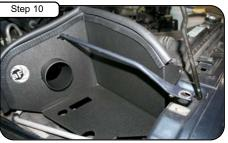
Attach trim seal to housing and install. Make sure core support bracket slides through hole on housing.
