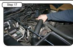
Attach straight coupling with #044 clamps provided on end of intake tube and position to housing and throttle body.
