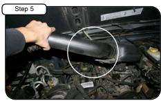
Pull crank case line away from stock intake and remove from vehicle.
