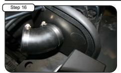
Attach elbow coupling with #048 clamps to housing and position. Do not tighten.
